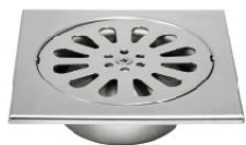
FD-4301 Stainless Steel 4" Floor Drain • Drain Rate 10 liters/minute • for 2" PVC Pipe
