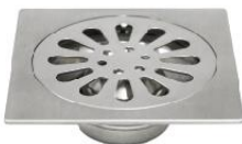
FD-4303 Stainless Steel 4" Floor Drain • Drain Rate 10 liters/minute • for 2" PVC Pipe
