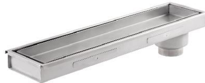
TSD-400T Stainless Steel Shower Drain with Tile Insert Grate • Length 40 cm. • with Frame • Drain Rate 25 liters/minute • for 2"-2.5" PCV Pipe
