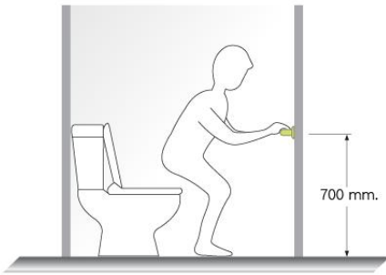
Horizontal grab bar installation in front of toilet
