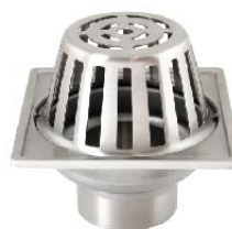
RD-4320 Stainless Steel 4" Roof Drain • Drain Rate 40 liters/minute • for 2" - 2.5" PVC Pipe
